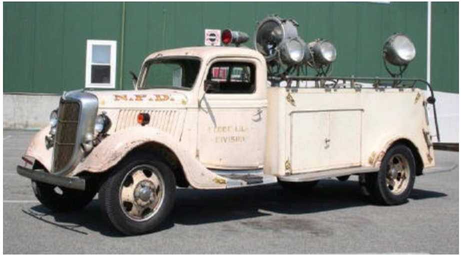
1936 Ford Floodlight rig with body built by Wendel Body Co of Newark NJ. Purpose built to bring ‘daylight’ to fire scenes, this rig was eventually retired from service as new apparatus were delivered with their own more powerful lighting equipment. Photo courtesy Ron Jeffers)
